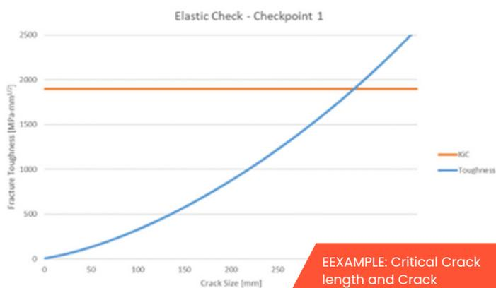
EEXAMPLE: Critical Crack length and Crack Propagation Pattern analysis (example on Gamesa G47)
